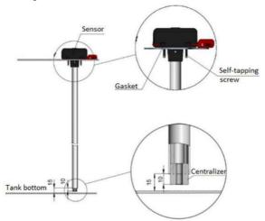
ANNEX 6. Methods of sealing of sensor head and cable connection
