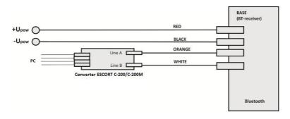
ANNEX 2. Wiring diagram of sensor base connection in RS-485 mode
