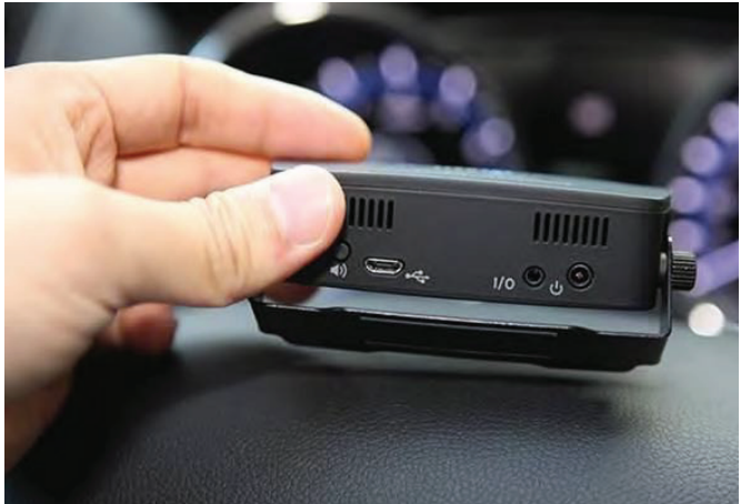
▲ This cradle has a guide that allows you to adjust height up and down after installation.
