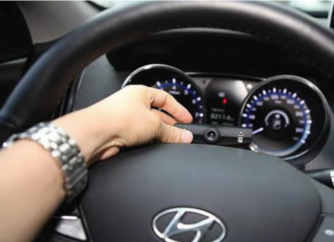
▲ This picture shows the product installed at the steering column cover.
