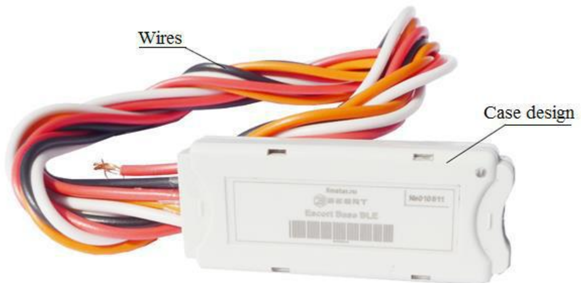
Fig. 3.2. BLE-BASE wireless capacitive fuel level sensor base design
