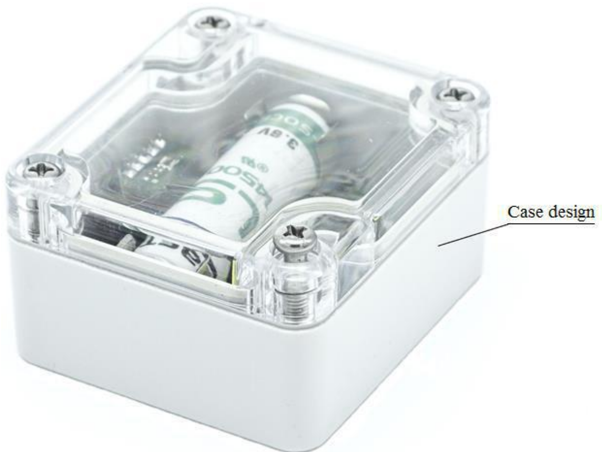
Fig. 3.4 TL-BLE Wireless temperature and light sensor design
